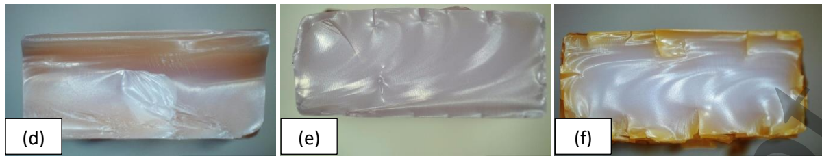
Fig. 7. Optical microscopy images of the cross-sections after break of the improved samples. (a) SLA-e as-printed; (b) SLA-e after 85 °C; (c) SLA-e after 185 °C; (d) SLA-g as-printed; (e) SLA-f as printed; (f) SLA-f after 185 °C.
