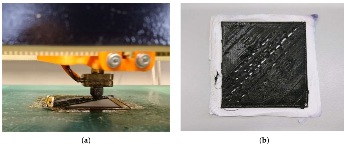
Figure 3. 3D printing squares of dimensions 40 mm × 40 mm on nanofiber mats previously dipped in soap water: (a) rough surface for a too large distance between nanofiber mat and printing nozzle; (b) 3D printed layer with uneven surface and even several not closed areas near the diagonal, i.e., along the longest lines, due to a too large distance between nozzle and nanofiber mat.
