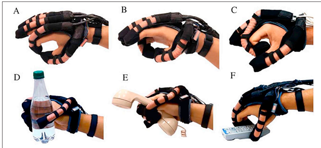
Figure 1. Soft robotic glove in diverse movements and grasping situations: A) index finger-thumb opposition contact, B) small finger-thumb opposition contact, C) index finger flexion, D) grasping a bottle of water using all fingers, E) picking up a telephone using all fingers, except of the small, and F) grasping of a television remote control using a tripod pinch. From a previous study 33 reprinted with permission from Elsevier.
